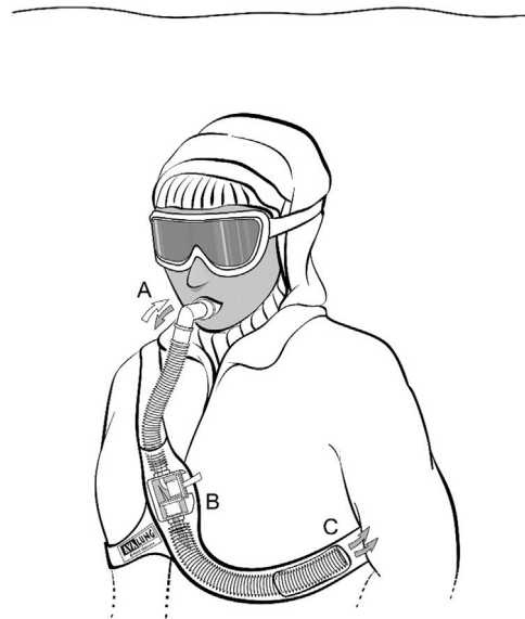
Figure 3. The artificial air pocket device that diverts expired air away from inspired air during avalanche burial is intended to prolong survival of fully buried avalanche victims. The white arrows show the flow of inspired air, and the gray arrows show the flow of expired air.
